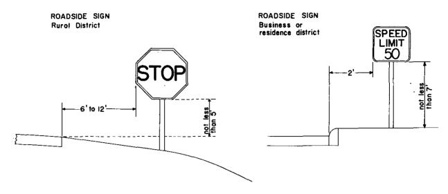
Figure 38. Examples of erection of temporary signs.
