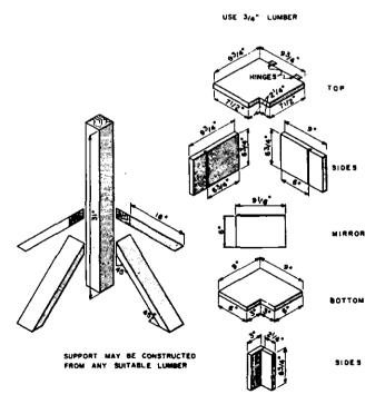
Figure 27. Dimensions of a mirror box.
