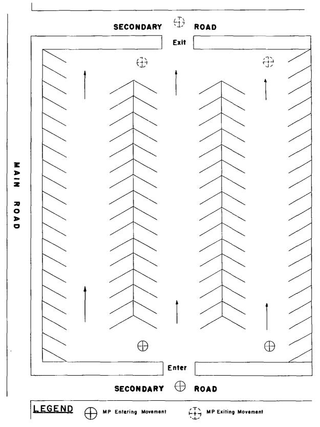
Figure 35. Example of a temporary parking facility with turnover. (See figure 6 for dimensions.)
