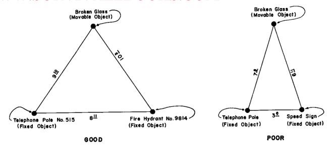
Figure 31. Example of triangles apex angle.
