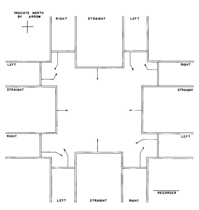
Figure 11. Field sheet for study of traffic volume and movements.
