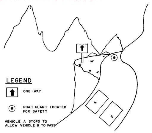
Figure 68. Example of vehicle passing on a narrow mountain road.
