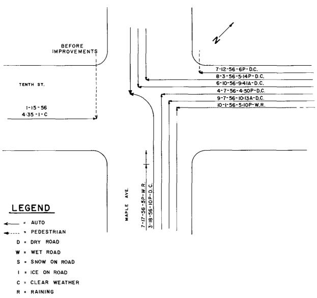
Figure 15. Sample collision diagram.
