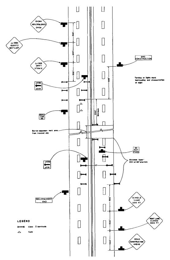
Figure 43. Example of a cross over on a 4-lane high speed road.
