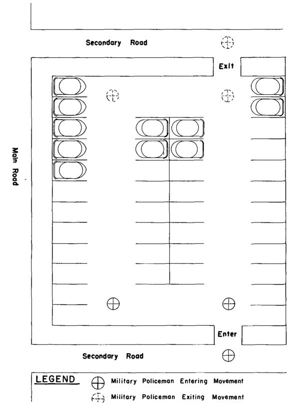
Figure 34. Example of a temporary parking facility with no turnover. (See figure 6 for dimensions.)
