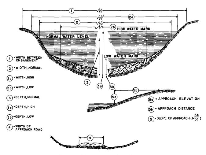
Figure 133. Standard dimensional data for fords.
