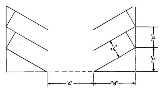
Figure 6. Dimensions for parking stalls.
