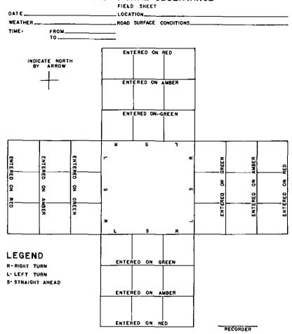
Figure 14. Sample field sheet for traffic signal observance study.
