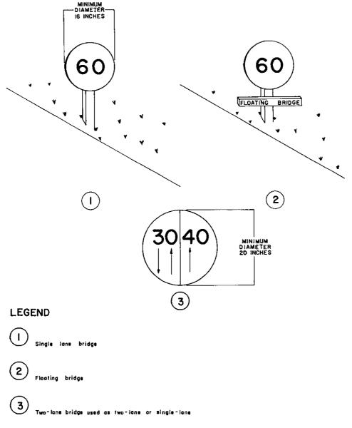
Figure 61. Example of bridge classification signs.
