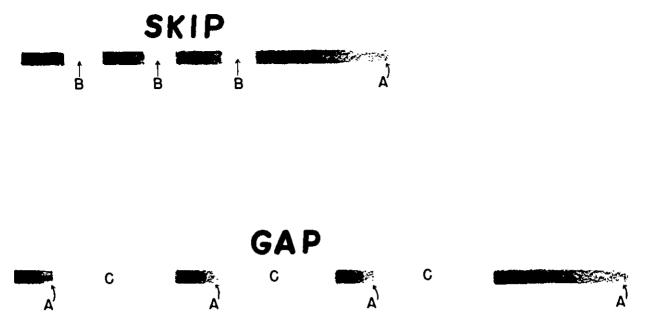
Figure 33. Skidmarks showing a gap and a skip. A—The shadow or light beginning of a skidmark; B—the skid between the skidmarks. Note the lack of a shadow or light skidmark after a skip. The distance of a skip is usually not more than 3 feet. C—The gap is an area where the brakes are not locked. The skidmark after a gap is a new skidmark starting with a shadow and light skidmark. The gap is usually in excess of 10 feet.
