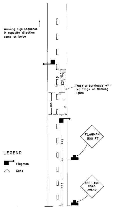
Figure 41. Example of one lane closed road using a flagman.
