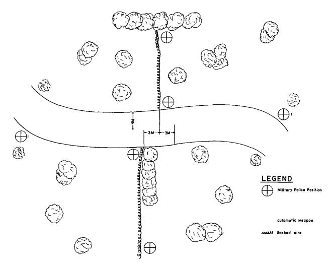
Figure 59. Example of a type roadblock.
