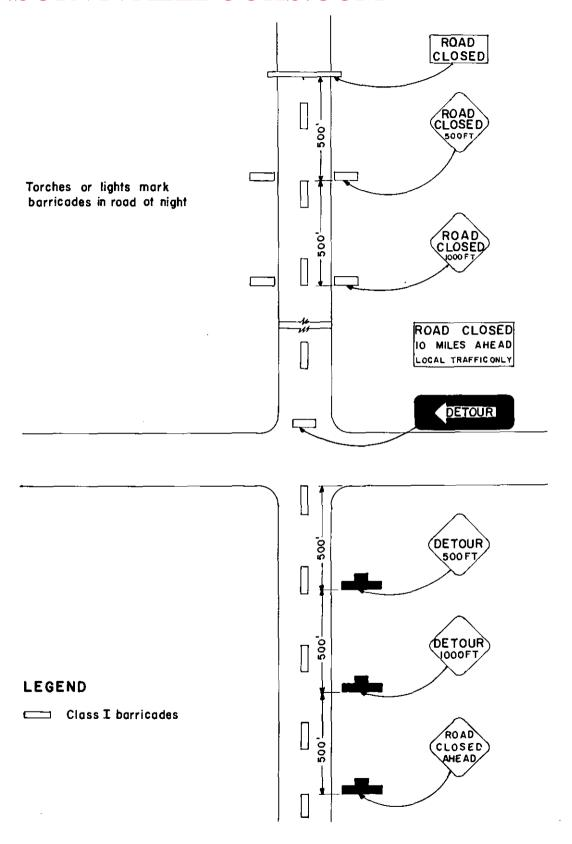
Figure 40. Example of signing for a closed road.
