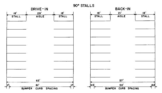
Figure 4. Minimum dimensions for parking area layout 90° stalls. (Minimum stall width for employee is 8.5 feet. Width of 9.0 feet should be used for visitor spaces and 9.5 to 10.0 feet for commissary and PX customers parking.)
