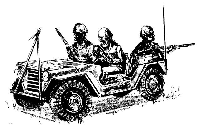
Figure 55. Example of a 4-ton vehicle with a deflecting bar.
