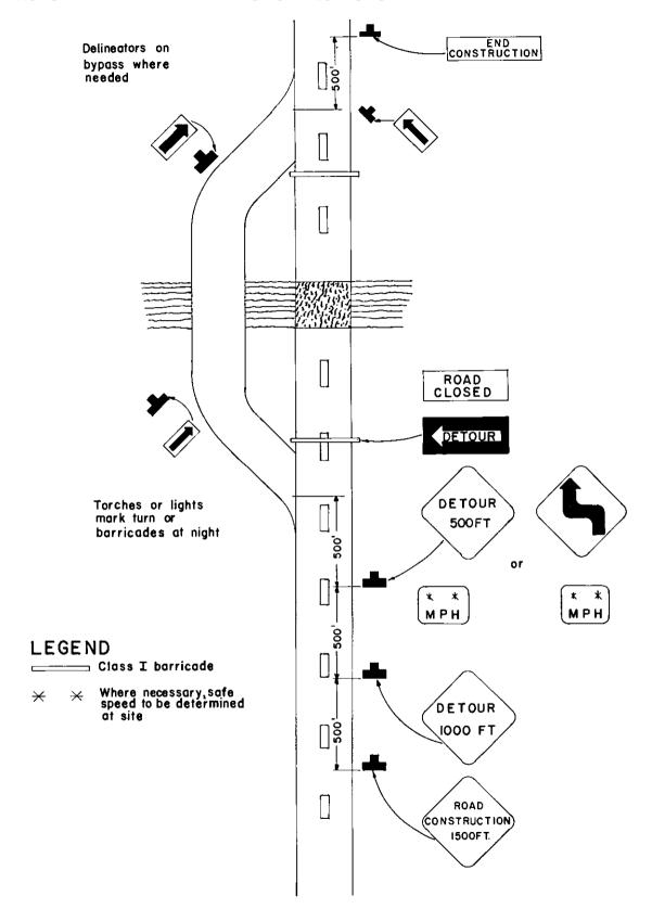
Figure 42. Example of signs used for a bypass road.
