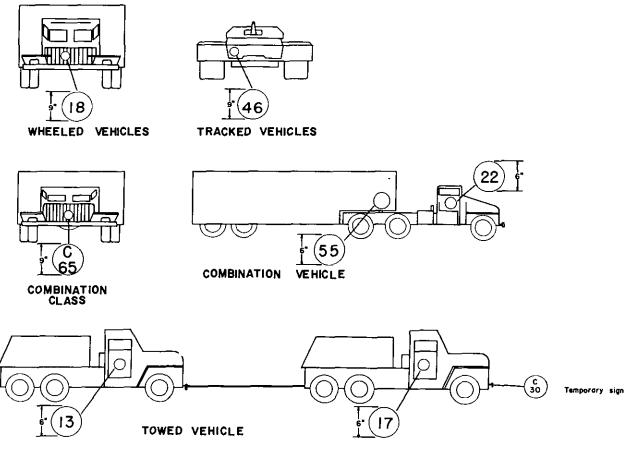
Figure 62. Example of methods of portraying vehicle classification.
