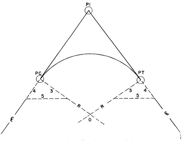
Figure 121. Curve radius by locating center of circle.
