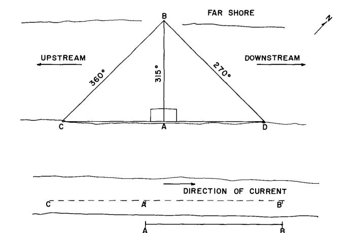
Figure 134. Methods of measuring stream width and velocity.
