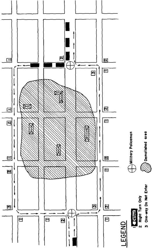
Figure 46. Example traffic rerouting.
