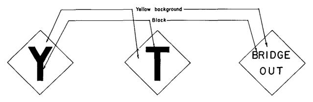
Figure 70. Hazard signs not provided for by the Geneva Convention.
