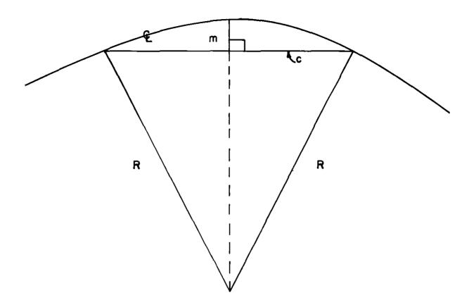
Figure 122. Measuring a curve using formula  $R = C^2/8m + m/2$ .
