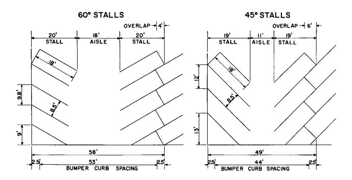
Figure 5. Minimum dimensions for parking area layout 60° stalls and 45° stalls (with stalls width of 8.5 feet.)
